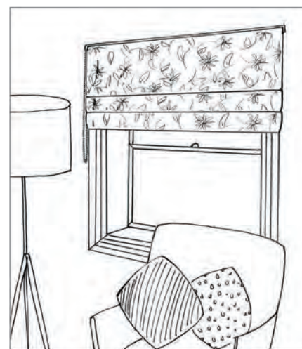
C - Fixed to wooden window architrave
